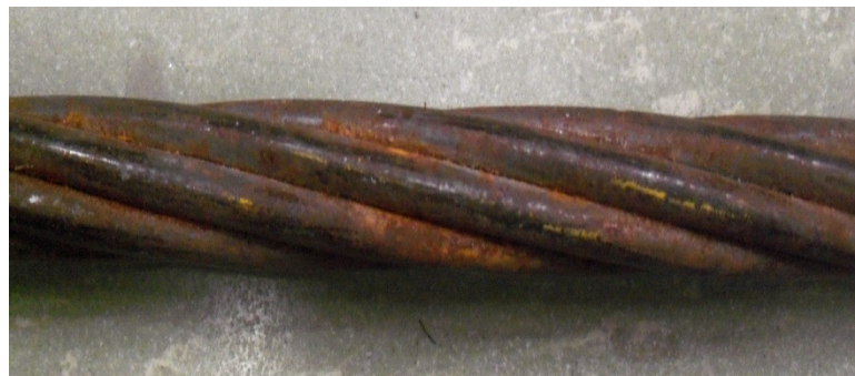
Figure 5.17 A 7-wire strand with no flaws used for baseline measurements.
