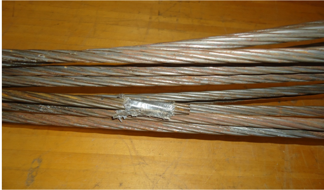
Figure 5.30 One-broken strand defect at the anchorage area.
