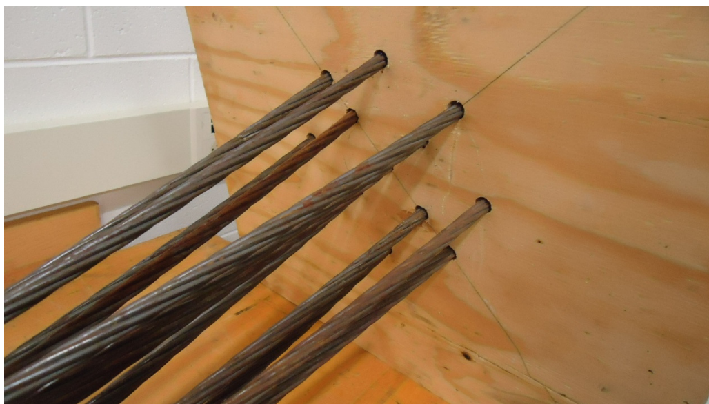
Figure 5.28 13-fan-out strands anchorage area.
